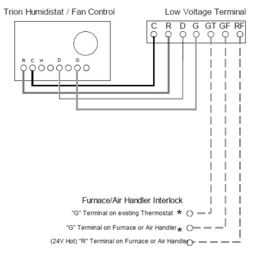
\* Remove Existing Wire Between T-stat "G" and AH/Furnace "G"
