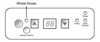
Figure 5. Dehumidifier Control Panel
