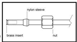
brass insert into the end of the plastic tubing.
