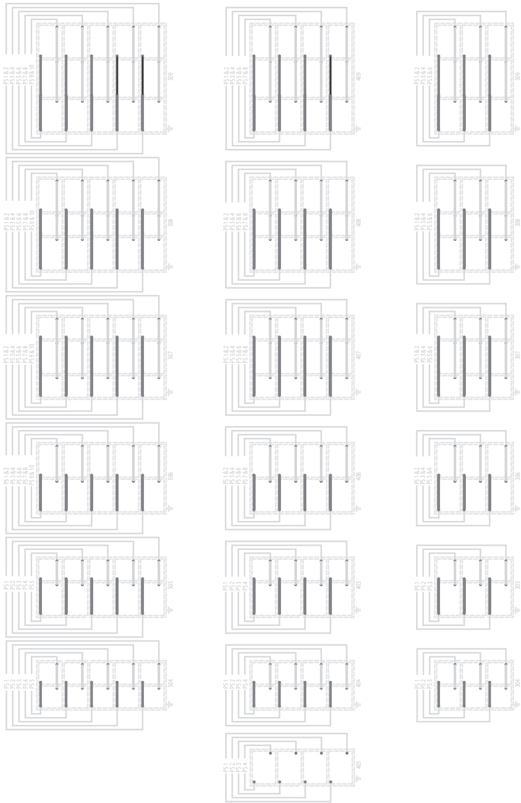
CELL ARRANGEMENT & BUS BAR CONNECTIONS MODEL 60-XXX-00 & 01
