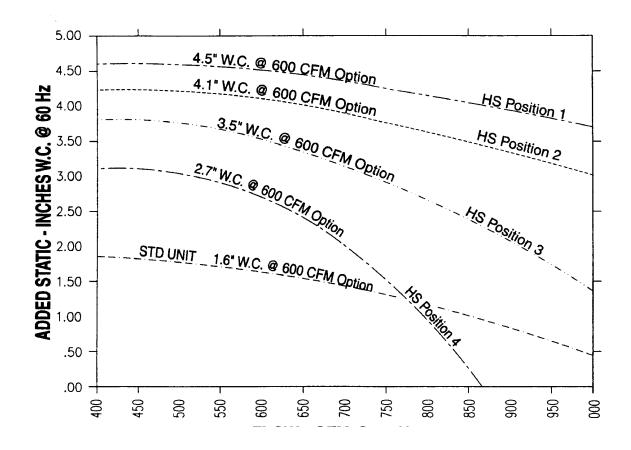
Figure 9 – System Performance Curves (without Filters)
