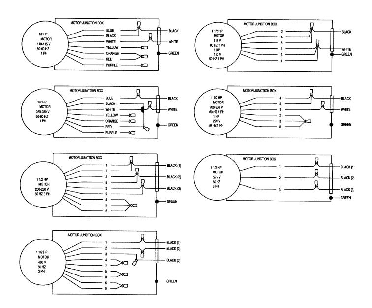
The MP600M is wired directly from the power source with 20 amps minimum, service utilizing 3 wire grounded cable, (115-208-230-460-575/60/3) for single 208-230/60/1, phase service and 4 wire grounded cable for 3 phase service, routed through appropriate conduit (See figure 5 wiring diagram). All wiring must be connected in accordance with local electrical codes.
