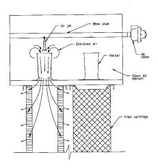
FRED<sup>TM</sup> SR C6 and C9 dust collectors are designed for the removal of dust or smoke from industrial applications. All models are equipped with a fully automated self-cleaning system and equipped with a high performance backward inclined blower.
