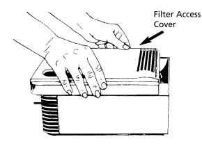
Install the Charcoal Filter on this side of the Filter Assembly, with the white side facing the electronic filter and the blue side facing out.
