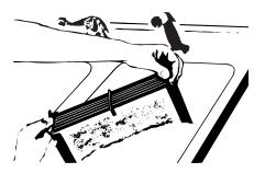
After the Electronic Filter has soaked sufficiently, agitate the cell up and down in the soaking solution until clean. If the Electronic Filter is extremely dirty, spray it with a common household cleaner or Electronic Air Cleaner solution. Allow the filter to soak for five additional minutes before proceeding with the rinse instructions.
