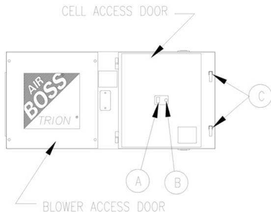
**Control Switch (A):** The control switch is located on the cell access door. It controls the operation of the power pack (and the belt driven blower on the T1300 and T2600). The control switch should be in the "OFF" position when the cell access door is open for maintenance of the unit.
