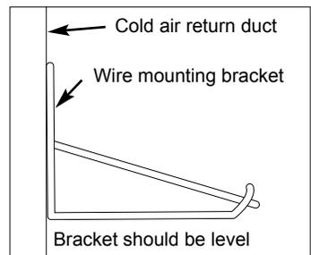
12. The discharge dome should approach the opening in the duct, however, it should not extend into the duct. There will be no heat loss, due to the negative pressure of the cold air return duct (the air flow will create a vacuum in the duct).
