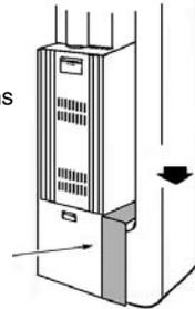
**Space Saver Furnace (Highboy)** – Side installation. Mounted vertically, where return air enters side inlet of furnace.
