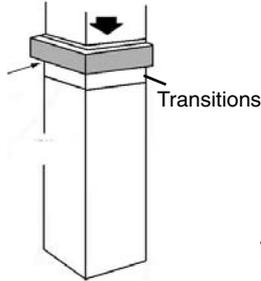
**Counterflow Furnace** – Mounted horizontally in return duct – just above the furnace.
